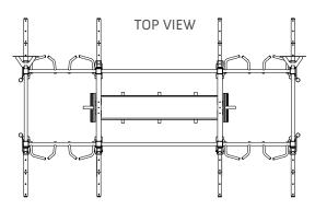
Note: Accessories shown are not included; X-Racks are required to be bolted to a concrete sub-floor
